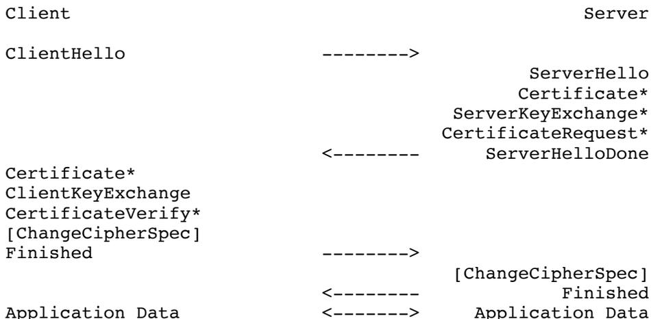
Fig. 1 - Message flow for a full handshake
