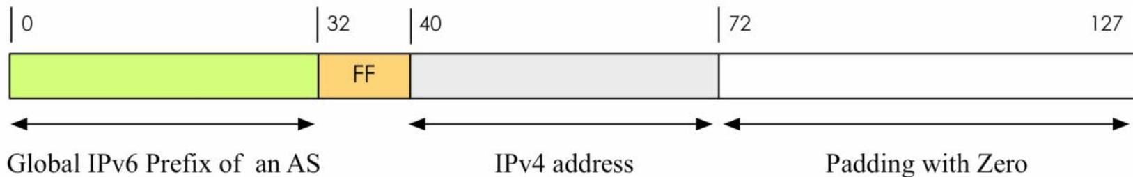
**Mapping Rule:** IPv4 addresses are embedded from bit 40 to bit 72 of the IPv6 addresses of a specific /32.
